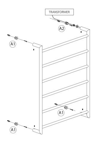
**A1** indicates brackets which fix the towel rail to the wall. They are installed using METHOD 1 as shown.
