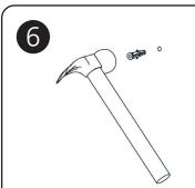
Hammer a wall plug into each base plate fixing hole that has been drilled.
