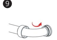
Carefully slide end covers back along the rail to each base plate and screw down securely.
