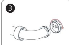
Unscrew the base plates from the fixing nuts and set aside the grab rail.
