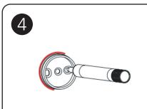
Put the base plates back in position according to the wall outlines. Mark each fixing screw hole location.
