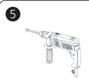
Drill 8 mm Ø holes to a depth of 70 mm at each marked screw location point.
