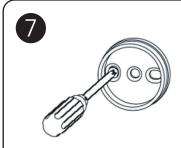
Tighten the screws, making sure the base plates are firmly secure and cannot move. Seal screw fasteners using a neutral-cure silicone sealant.
