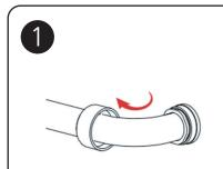
Unscrew all end covers from their base plates and carefully slide them along the rail away from the fixing plates.
