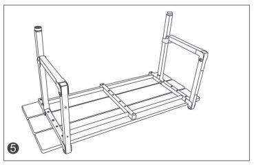
Place assembled seat on the wall in the required location. Check the seat is level front to back and left to right. The top of the seat must be 460-480mm from the finished floor. Mark screw hole fixing locations on the wall.
