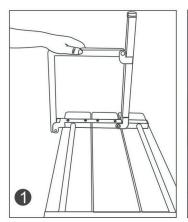
Place seat (A) upside down on a flat surface. Open leg (B) and locate on back of seat.
