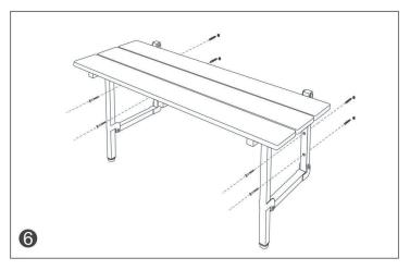
Drill 8 mm  $\varnothing$  holes to a depth of 60 mm at each marked screw location point. **NOTE** Use an appropriate drill bit for the wall material. Place wall plugs into holes.
