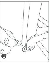
Insert nylon gaskets (C) into gap between leg and seat frame.
