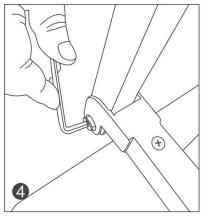
Use Allen key (F) to tighten bolt (D). Repeat for second leg. **NOTE** Do not overtighten bolts.
