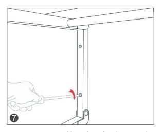
Reposition seat assembly on the wall and secure with fixing screws provided (E). Seal screw fasteners using a neutral-cure silicone sealant.
