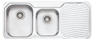
PE311 (Left hand bowl) PE312 (Right hand bowl) 1080W x 480H x 180D MAIN BOWL 21 LITRE / \frac{1}{2} BOWL 11 LITRE
